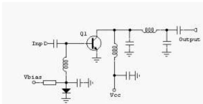
A single transistor may be used in a Class-B configuration. The only requirement in this case is that a resonant circuit must be placed in the output network of the transistor in order to “reproduce” the other half of the input signal.
