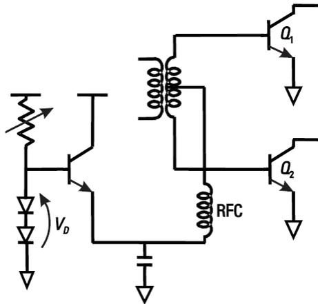
In the above example, all diodes and transistors are assumed to be at the same temperature. As temperature rises,  $V_D$  falls, reducing  $V_{BE}$  and keeping  $I$  constant.
