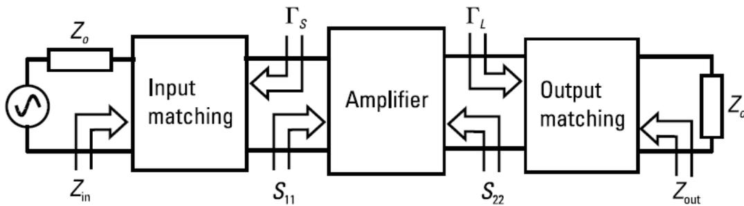
If matched:  $Z_{in} = Z_o$ ,  $\Gamma_s = S_{11}^*$ , and  $Z_{out} = Z_o$ ,  $\Gamma_L = S_{22}^*$
