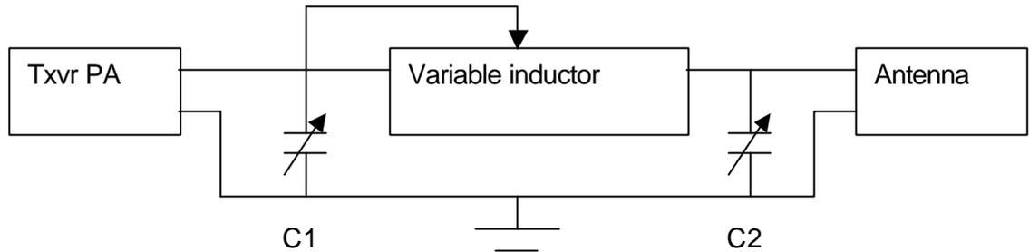
The two capacitors, C1 and C2, act as impedance splitters and conjugate matchers. Imagine the two Cs disconnected from ground – they are now in series and have an L in parallel – ie, we have a parallel LC resonant tank. Our aims are to adjust this tank for
