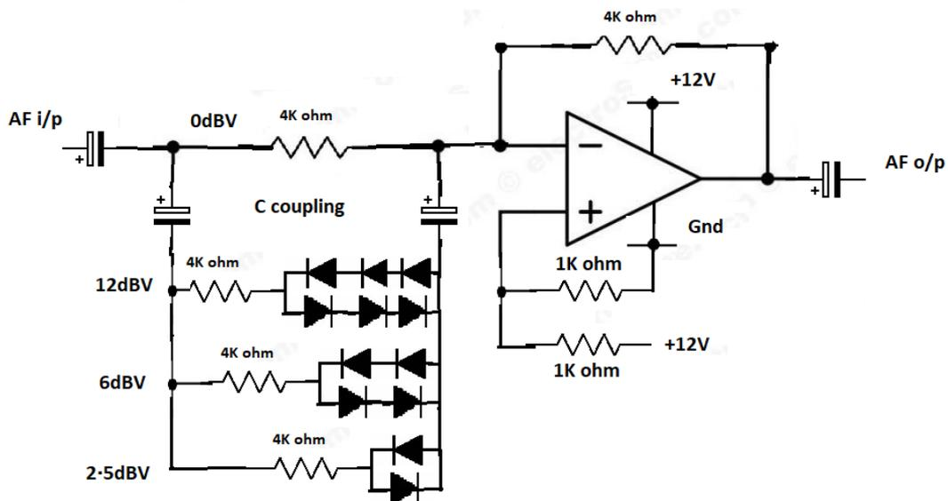
Now to be honest, while yes, I had to redesign the logarithmic circuit, and behind the scenes to this design are the mathematical models to prove the compression curve, using both just the op-amp gain equation. Here too by replacing the 4Kohm feedback resistor with a variable adjustment
