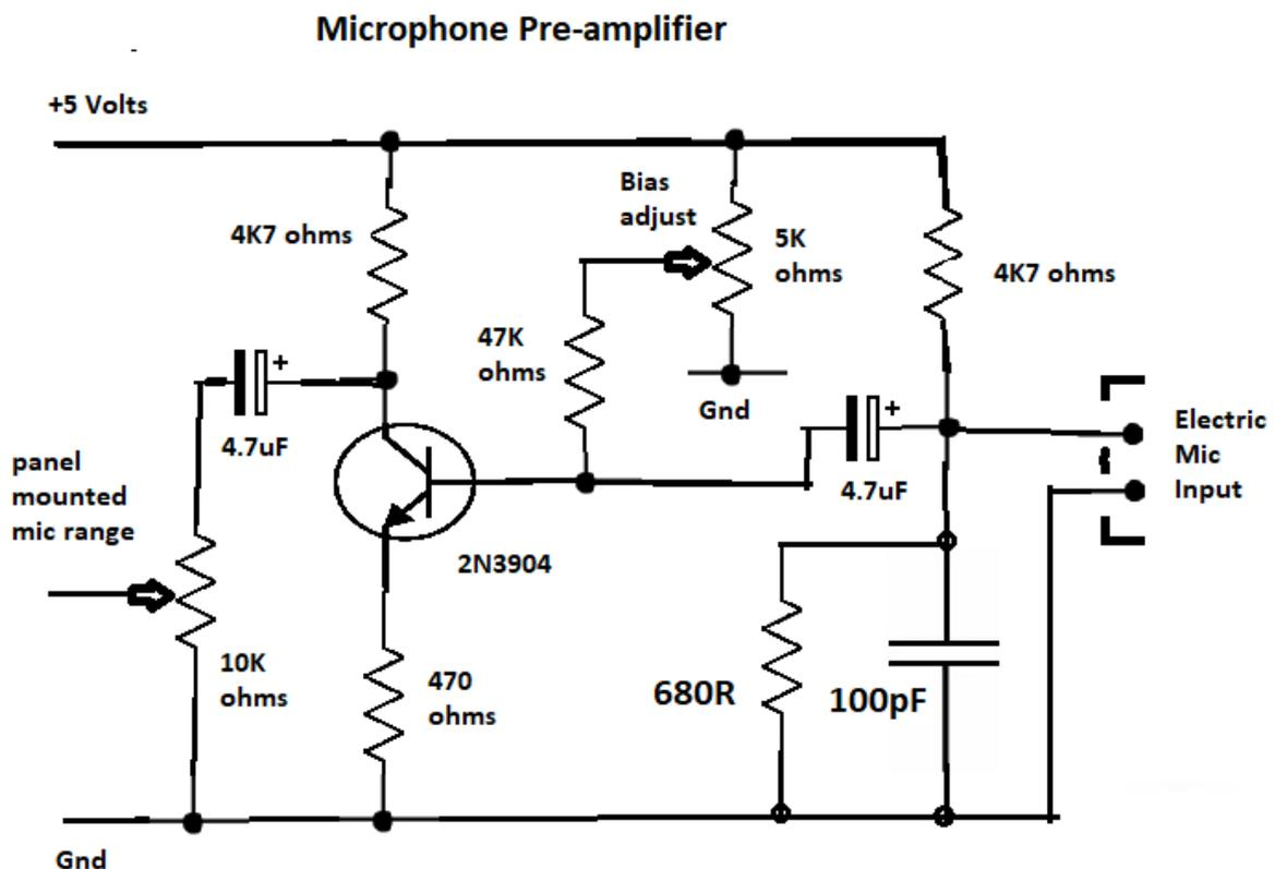
A mid stage audio amplifier was found to be required, so the below circuit has been constructed for the microphone audio amplification, a mid-stage amplification trim is used, setting the overall max level of voice audio signal gain, shown below:
