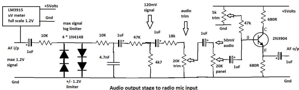
Using the above circuits, an audio compressor circuit can be simply constructed. I have completed my own construction, just using the 5Volt supply from my FT450d microphone connection.
