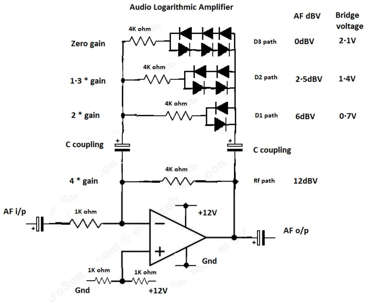
The addition of the “C coupling” capacitors, is to provide a ground voltage reference for the diode feedback circuit to function.
