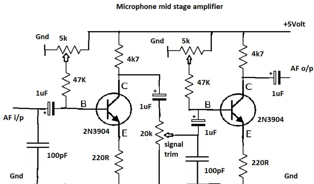
The emitter circuit DC bias setting across the emitter resistor, does not use a by-pass capacitor for an AC signal gain setting. It was found that the capacitive reactance of the emitter capacitor, shunted the DC bias current, thus causing audio distortion within the audio signal. The higher the sound signal frequency, the worse the problem became.
