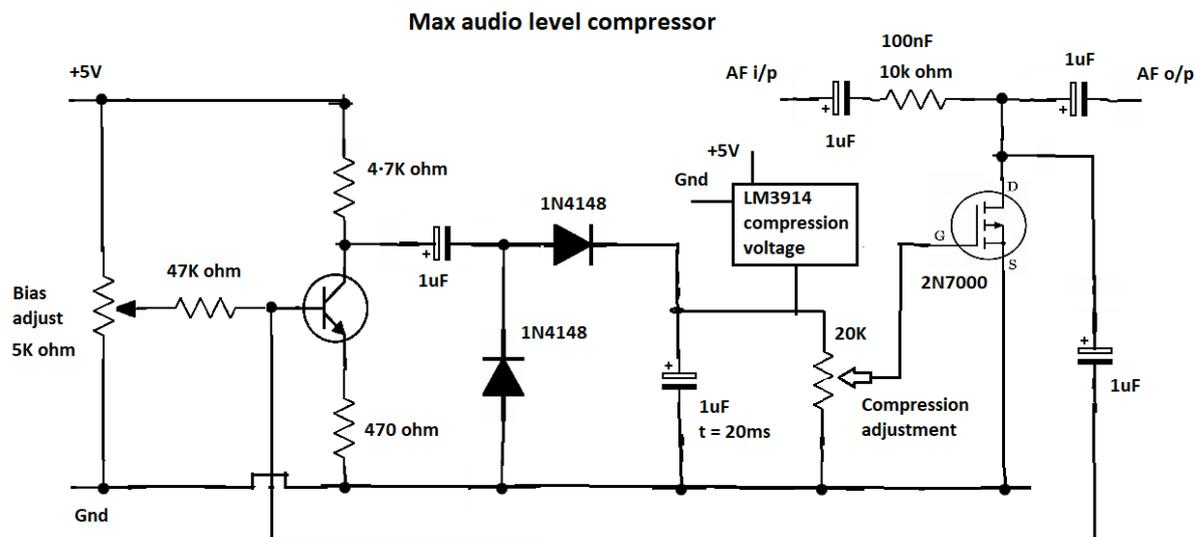
A max audio level compressor, once the spoken voice audio peak above a minimum limit, the automatic gain control adjustment will reduce the audio amplitude, by virtue of the 20k ohm variable and the mosfet 2N7000, half "T section" attenuator circuit.
