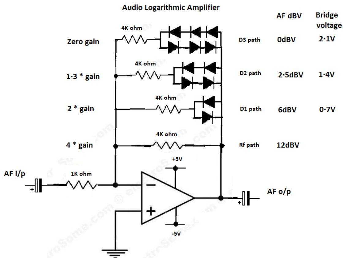
As each bridge voltage is breached, an additional feedback resistor comes into play, creating a parallel resistance with resistor “Rf”, the 4K ohm resistor to give the four times original signal gain.
