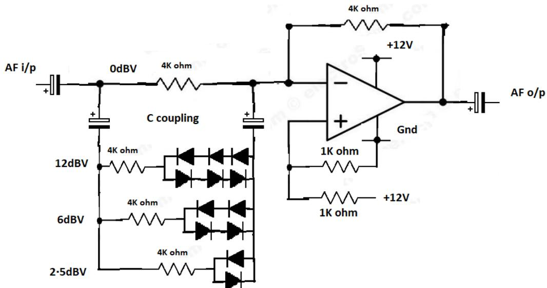
Now to be honest, while yes, I had to redesign the logarithmic circuit, and behind the scenes to this design are the mathematical models to prove the compression curve, using both just the op-amp gain equation.
