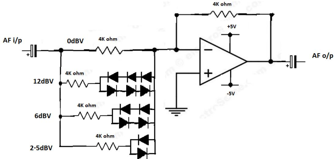
For the logarithmic expander circuit, it is perhaps best to use Shockley diodes due to their low forward voltage, otherwise referred to as the “barrier potential” voltage.
