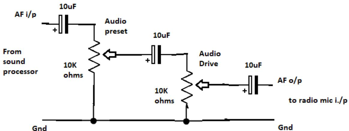
The audio pre-set control is placed upon the circuit board, but the audio drive is a front panel mounted control, allowing the overall transmitter signal wattage to be altered while using SSB mode. With SSB, the lower the audio signal, the lower the output signal power overall.
