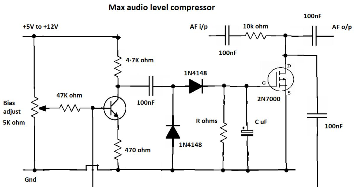
Notice however, that the spoken voice audio content below the limit threshold, is not affected by this circuit, as this part of the low level voice audio, its base level needs to be boosted up to bring up the low level audio signal.
