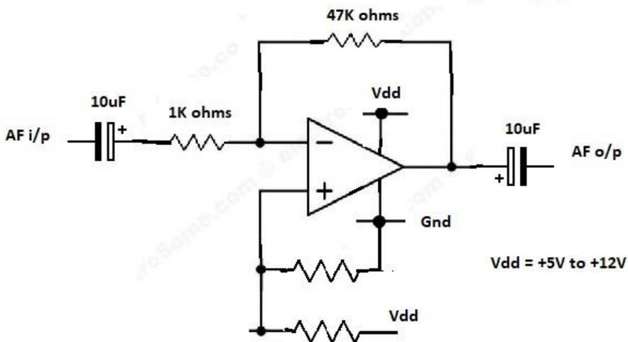
The main microphone amplifier has a signal gain of 47 times. With the combination of the microphone pre-amplifier, the overall microphone sound amplification is alterable from 47 times to 470 times.
