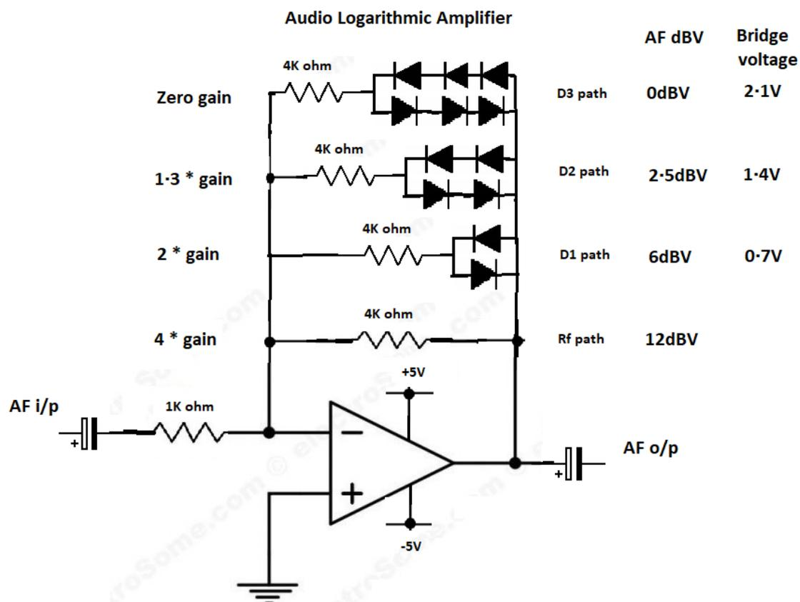
As each bridge voltage is breached, an additional feedback resistor comes into play, creating a parallel resistance with "Rf", the 4K ohm resistor to give the four times original signal gain. By changing the new bridge voltage resistor feedback values, a compression curve of one choosing can thus be created.
