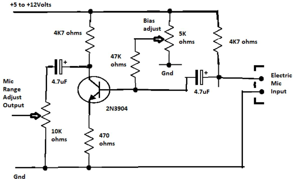
I discovered while searching with an oscilloscope, that while the DC bias was fine, as soon as a sound signal was sent through the sound amplifier circuit, the signal itself was in effectively altering the DC bias settings.
