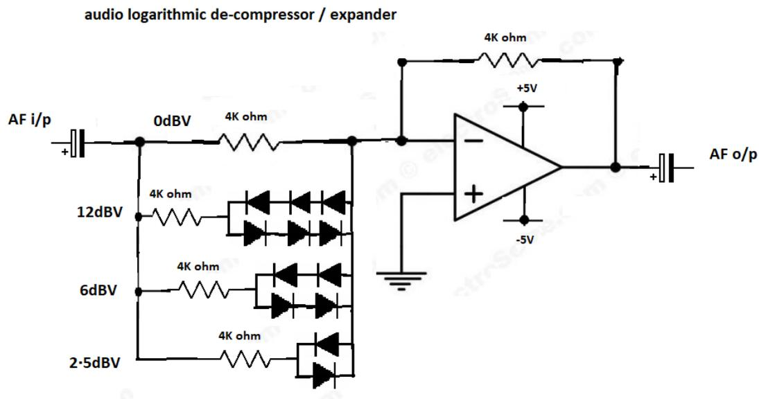
For the logarithmic expander circuit, it is perhaps best to use Shockley diodes due to their low forward voltage, otherwise referred to as the “barrier potential” voltage.
