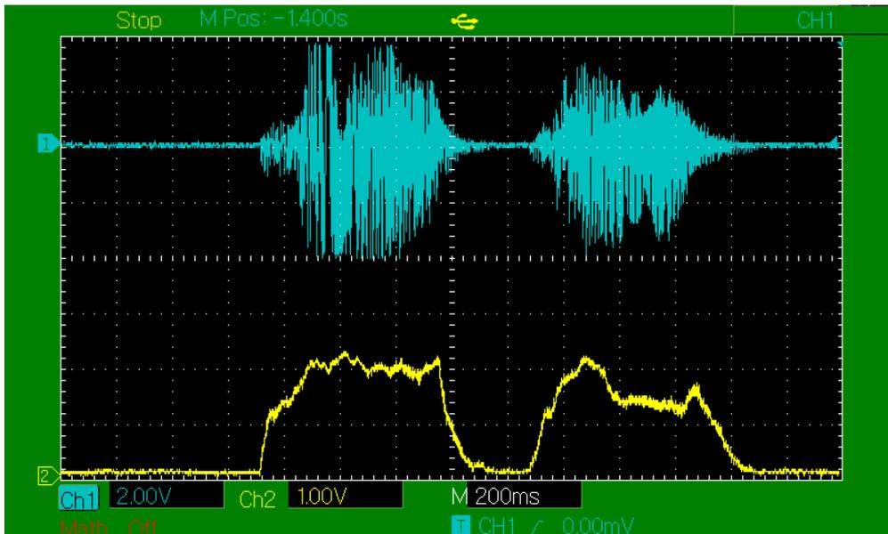
The principle test circuit can be used as a monitor sound test, by simple placing the microphone in front of the radio’s speaker.
