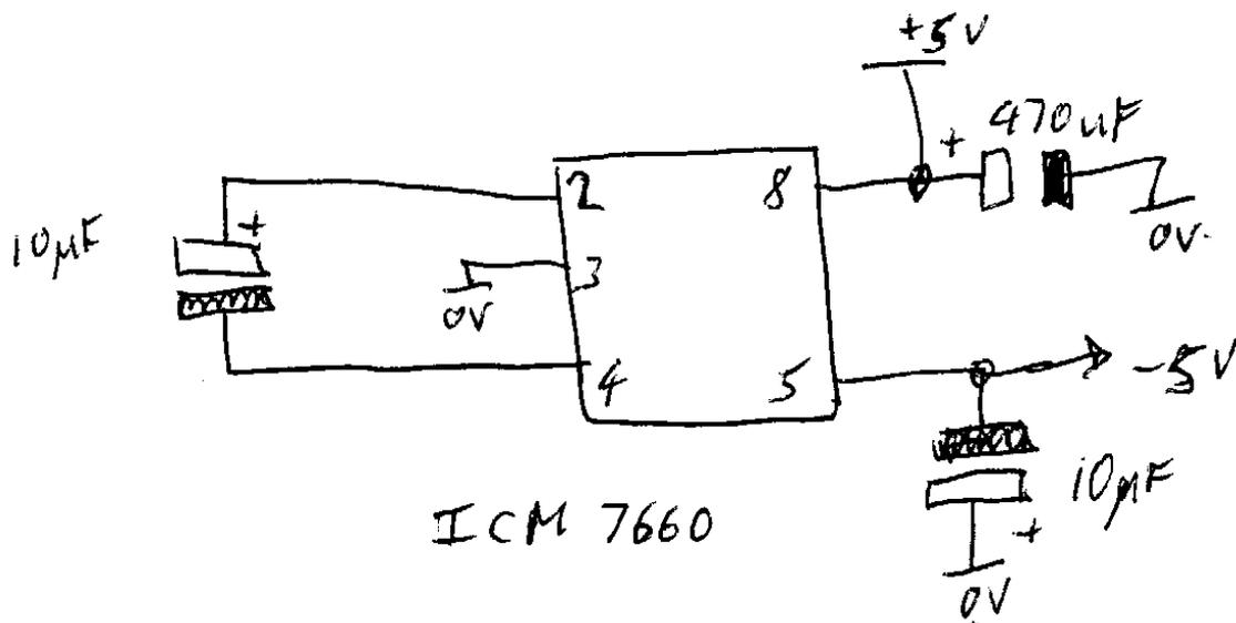
On first-hand the 5volt supply was sourced from a series of "AA" sized batteries, but I eventually dug out the variable voltage "psu" and used the 5volt supply output. However, I found that switching signals are present, so by adding a 470uF capacitor to the 5volt line, the disturbance was removed.
