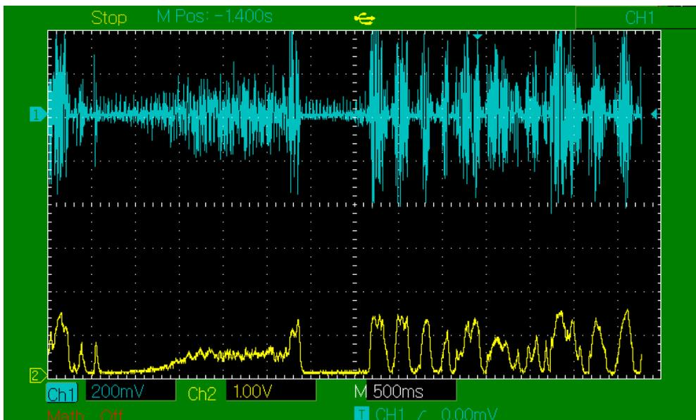
However, notice the gradual ramping of the yellow line to the left, as this is the radio’s agc response rebalancing the radio agc circuit voltage. The conclusion here, is that the modern radio’s use a reduce and then boost of the voice signal, in that there are using a constant volume amplifier circuit implementation. This then accounts for bouncing noise floor of the radio in noisy band conditions.
