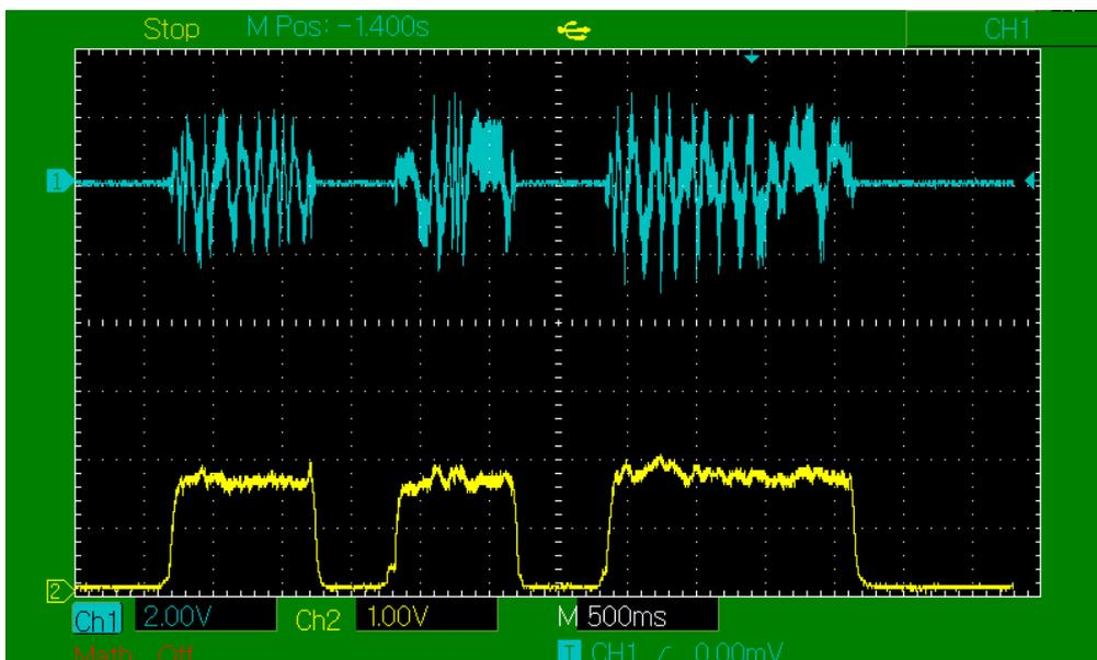
The next oscilloscope plot tracing are test wordings on the microphone, using the wording “hello” twice around.
