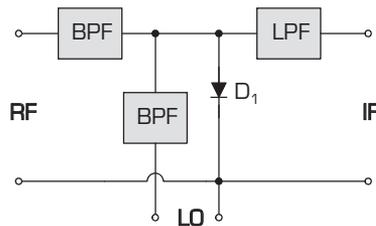
FIGURE 7.3 A basic single-diode mixer circuit with filtering.
