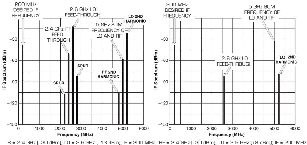
**FIGURE 7.10** Various single-tone mixer spurs generated by the single-ended mixing of the RF (2.4 GHz at  $-30$  dBm) and the LO (2.6 GHz at  $+13$  dBm), and their harmonics in an unbalanced mixer, with light one-pole filtering (left); a DBM diode mixer’s IF output spectrum in a well-balanced circuit (right).
