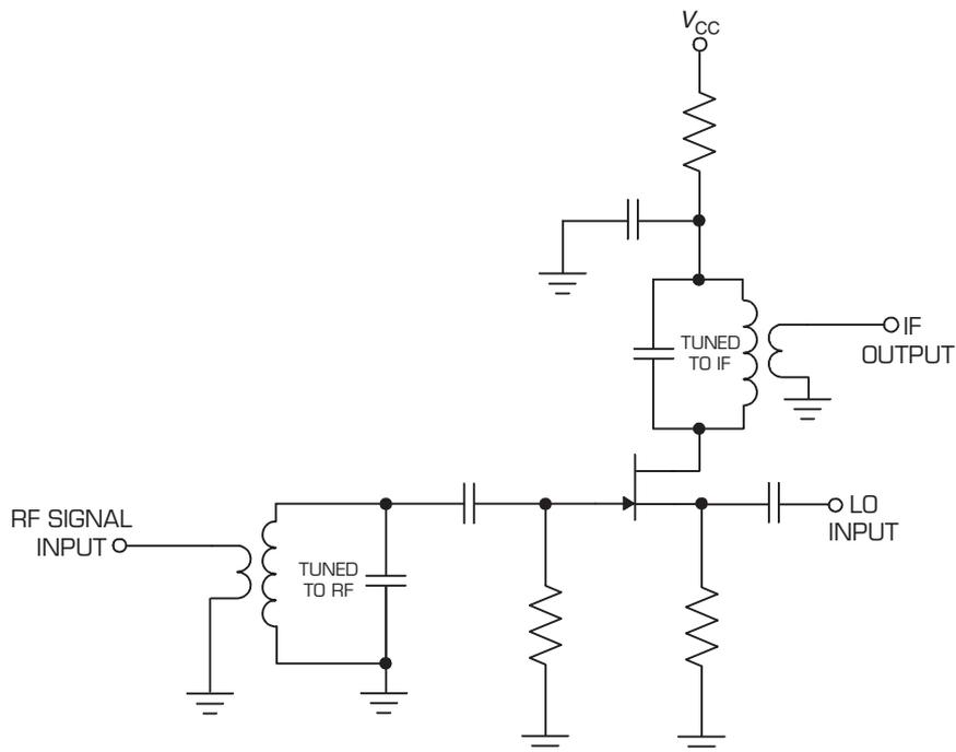
**FIGURE 7.13** A single-ended active JFET mixer circuit.
