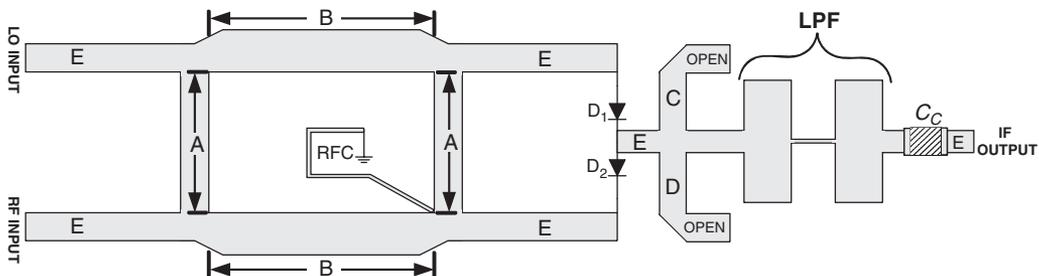
**FIGURE 7.7** A narrowband microwave mixer for UHF and above applications.
