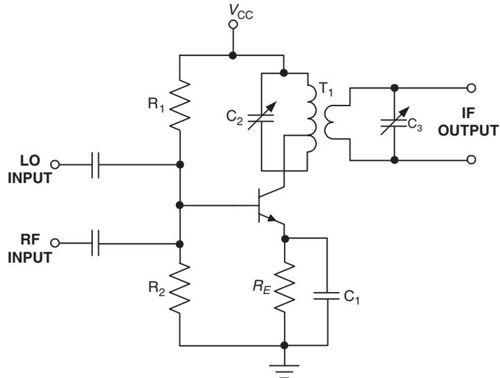
**FIGURE 7.15** One method of using a transistor as a nonlinear mixer stage.
