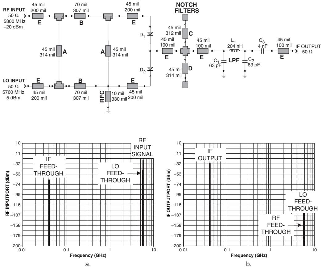
**FIGURE 7.8** The example single-balanced diode mixer circuit with calculated part's values, along with harmonic balance frequency sweep results (log scale): (a) All the signals present at the RF input port; (b) All the signals present at the IF output port.
