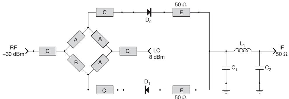
**FIGURE 7.9** The rat race distributed diode mixer circuit.
