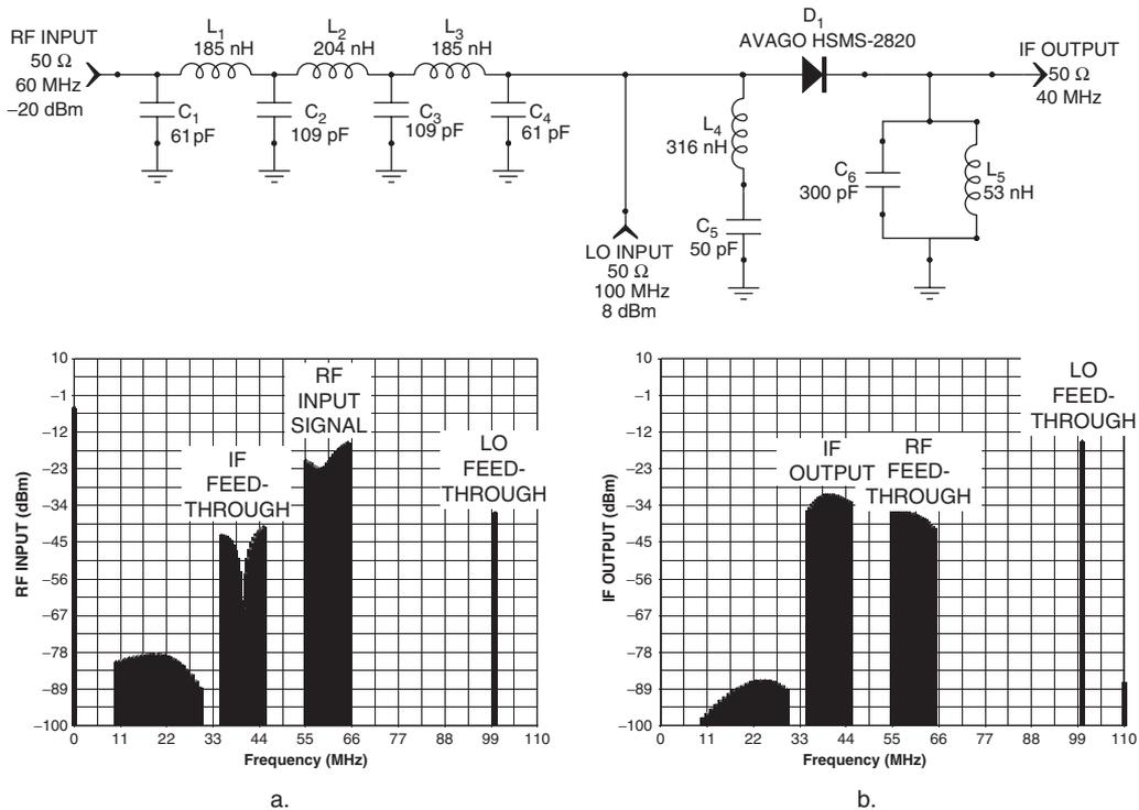
**FIGURE 7.6** The example single-ended diode mixer circuit with part's values, along with harmonic balance frequency sweep results: (a) All the signals present at the RF input port; (b) All the signals present at the IF output port.
