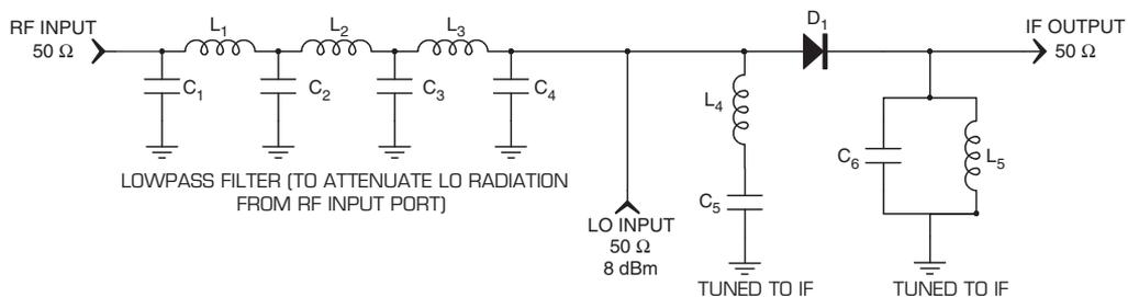
**FIGURE 7.5** A practical single-ended diode mixer circuit.
