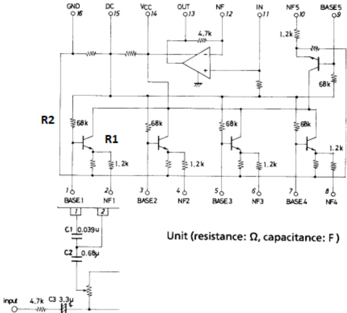
Assume that the input AF audio signal is used to excite the illustrated transistor stage into an RC tuned filter action. The degree of interaction depended upon the variable resistor wiper position, thus the audio input signal tap.
