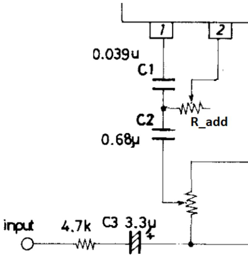
The additional series resistance, principally tunes the bandpass filter to the correct centre frequency, as required per the circuit application design specifications.
